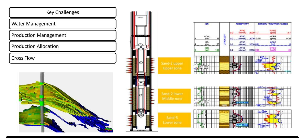
SW is 1st Subsea well completed in Mediterranean as a triple zone over Sand-2 Upper, Sand-2 lower and Sand-5
