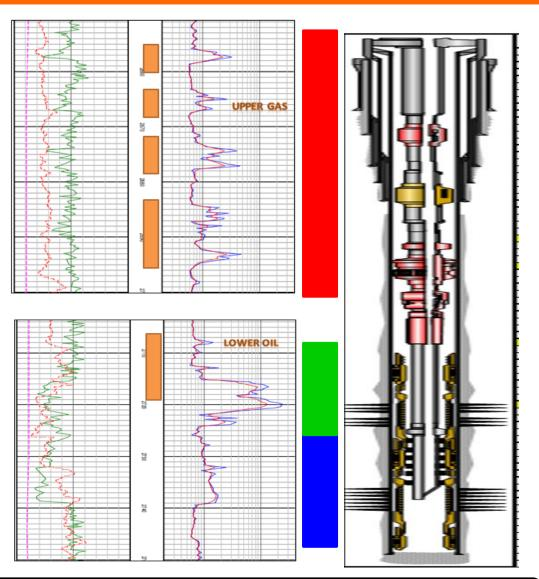
The well was completed as dual zone completion over gas zone(upper layer) and oil zone (lower layer).
